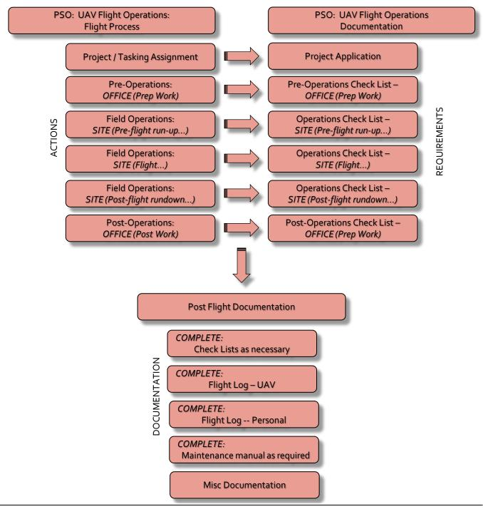
Graphic 04.01.01 – Procedure to conduct a flight operation.
